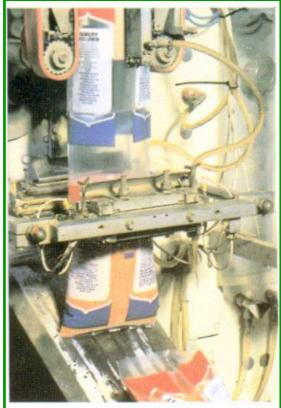
Used on the heated jaws of packaging machine to prevent sticky residue causing problems on bag sealing operation.
